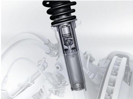
**PASM - Porsche Active Suspension Management** is the electronic damping (shock absorbing) control system. It actively and continuously regulates damping forces according to driving style and road conditions. In addition, the suspension is lowered by 10 mm. PASM has two modes, which can be selected using a separate button on the centre console: ‘Normal’, which is a blend of performance and comfort, and ‘Sport’ or “Sport Plus” where the setup is much firmer.
