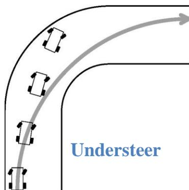
High slip angle at the front is known as Understeer (also push or tight in NASCAR terms). The car steers less than (or under) what the steering input is and is being pushed straight ahead.
