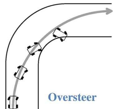
Usually, you can control understeering or oversteering conditions with the throttle. If you remember the Friction Circle, you know you have maximum steering capability using an even throttle (neither accelerating nor decelerating). Adding throttle shifts the weight to the rear, giving the rear better traction. Reducing throttle shifts the weight forward, allowing more grip in the front.
