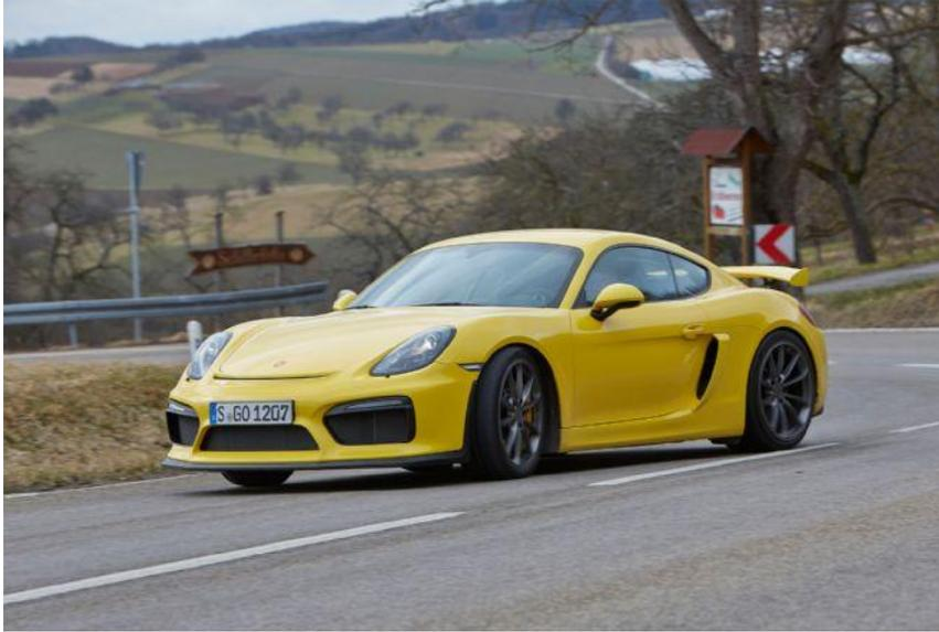
Here is a picture of a car that is oversteering. How do I know? Look at the road behind it. It is “S” shaped and the driver is negotiating a right hand turn. But if you look at the front wheels, the driver is steering to the left and not the right. You can tell the driver is on the throttle and not the brake as the nose of the car is raised. By keeping on the throttle, the rear tires have more grip even though they are sliding
